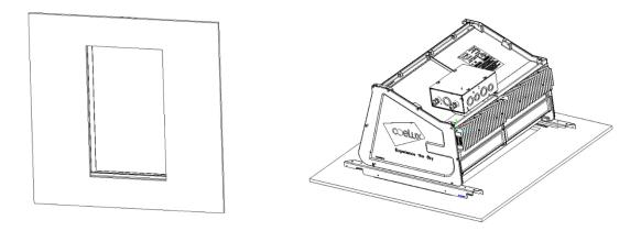
Fig. 13 Mounting for plasterboard false ceiling: step B.
