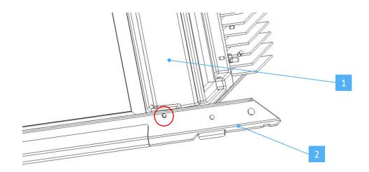
Fig. 4Detail of the support bars [2] for CoeLux ST (seen from below).Red circle: hole to fasten bars to the main case [1].
