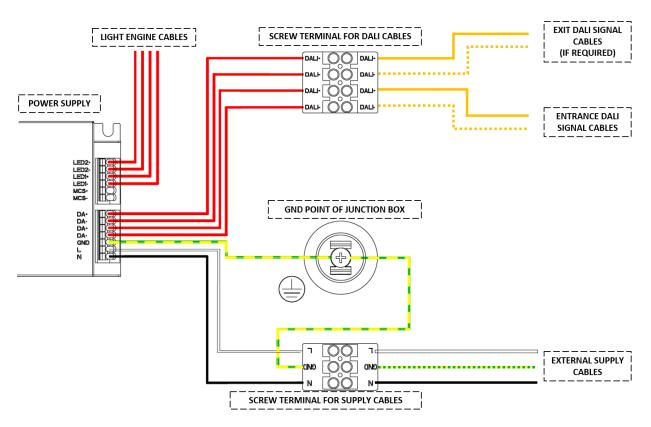
Fig. 20 Electrical diagram for connections with the external supply cabling and DALI.
